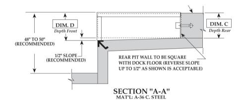
\*NOTE 1 : Angle 3"x3"x1/4"x20" Minimum Length or Run Continuous Pit to Pit. (Supplied By Others)
