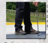
Conveniently located pull-chain provides easy activation of deck and lip.
